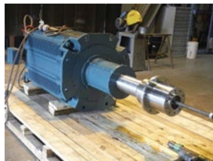
5. Fan motor of the permanent-magnet direct-drive type is ready for installation
