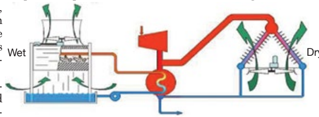
2. Typical wet/dry parallel condensing system
