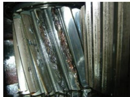
**11. Secondary pinion gear damage** suffered at Gateway Generating Station
