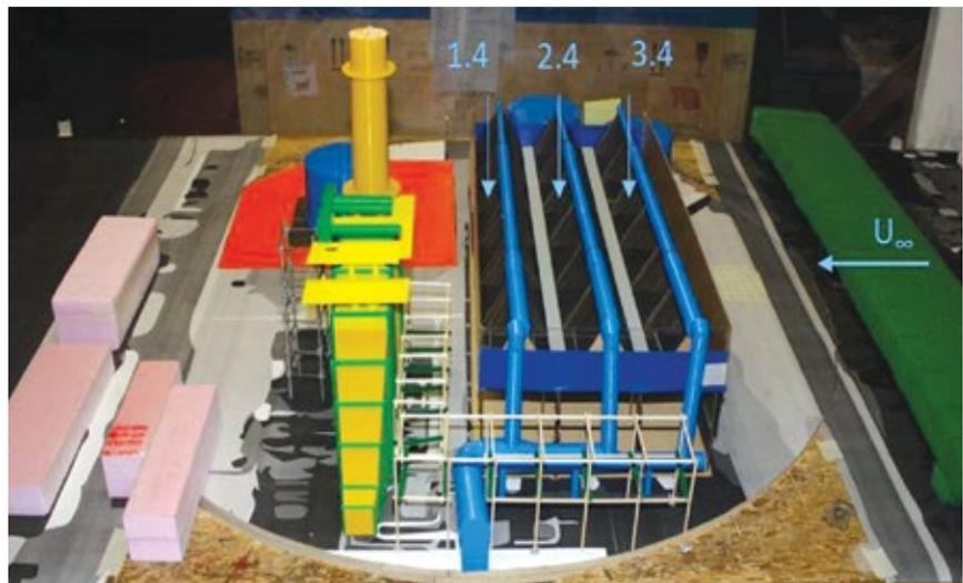
**17. A physical wind-tunnel model** was developed to advance the depth and breadth of the Caithness studies
