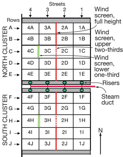
**27. ACC at NV Energy's Walter M Higgins Generating Station has 40 cells, arranged as shown. Note location of screens and their different configurations**
